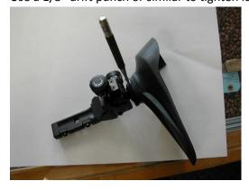
7) The Aperture Extension is also equipped with 1/8" holes so that a second drift punch may be used to keep it from counter-rotating while tightening the locking ring
